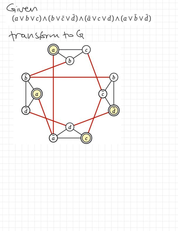
$(\underline{a} \vee b \vee c) \wedge (b \vee \overline{c} \vee \overline{d}) \wedge (\overline{a} \vee c \vee d) \wedge (a \vee \overline{b} \vee \overline{d})$ Transform  $(\overline{\Phi})$ : • make I triangle per clause · Connect inverses claim. D is satisfiable 2=7 G has an indep. Set of size k Proof: I is satisfiable. Fix a satisfying assn. Each clause has a T literal. Select one from each and add to a set Sis an IS.
